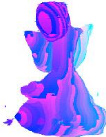
Computer's model rendered with triangle number as colour
